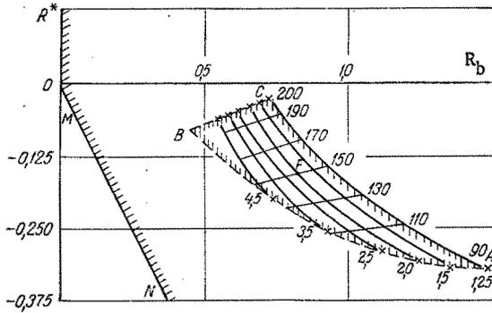
Fig. 1. Differential resistances of arc as function of resistance of ballast rheostat. ABC) stable arc region; MN) boundary. The figures on the line AB give the gas flow rate in  $\text{g} \cdot \text{sec}^{-1}$ ; those on the line AC give the current in A.  $R^*$  and  $R_b$  are in  $\Omega$ .
