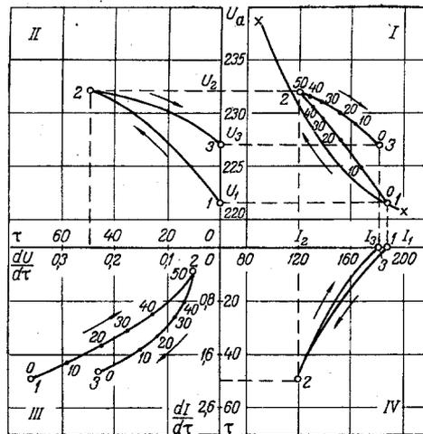
Fig. 3. Static and dynamic CVC of plasma-tron with interelectrode insert and distributed gas injection. The gas was air;  $G_g = 2.0 \text{ g} \cdot \text{sec}^{-1}$ ,  $d_a = 1.5 \cdot 10^{-2} \text{ m}$ ,  $d_c = 1 \cdot 10^{-2} \text{ m}$ ,  $d_s = 1 \cdot 10^{-2} \text{ m}$ ,  $n_s = 3$ . The solid line in quadrant 1 is the SCVC. The figures on the graph are the time in sec,  $\tau$  in sec,  $U_a$  in V,  $dU/d\tau$  in V/sec, and  $dI/d\tau$  in A/sec.
